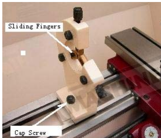
Figure 3. Steady rest in place.
