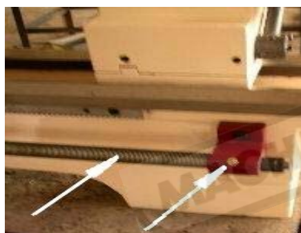
Figure 42. leadscrew bearing lubrication point
