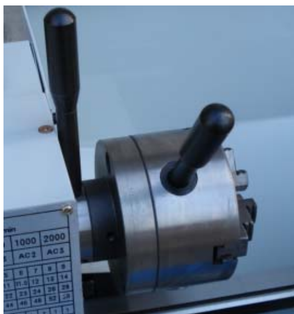
Figure 2 .Chuck removal bars in place
