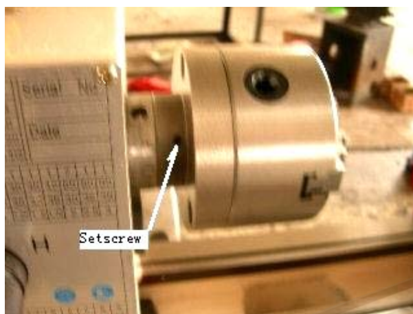
Figure 1 Typical chuck mounting .
