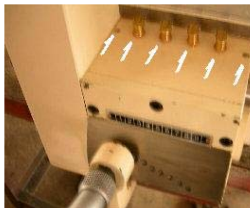
Figure 39. Gearbox lubrication caps and oil balls
